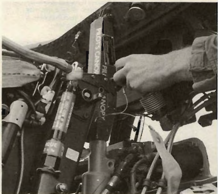
Installing canopy jury struts without inserting locking pin sets up a great booby trap. Upper: Strut can easily teeter forward against banana links. If canopy is closed from ground, or pressure drains off letting it lower, firing mechanism is inevitably damaged. And if Murphy has failed to insert safety pin, the seat gun will fire, though interlock remains in position. Below: Simply inserting jury strut pin may save crew chief embarrassment, and pilots life.
