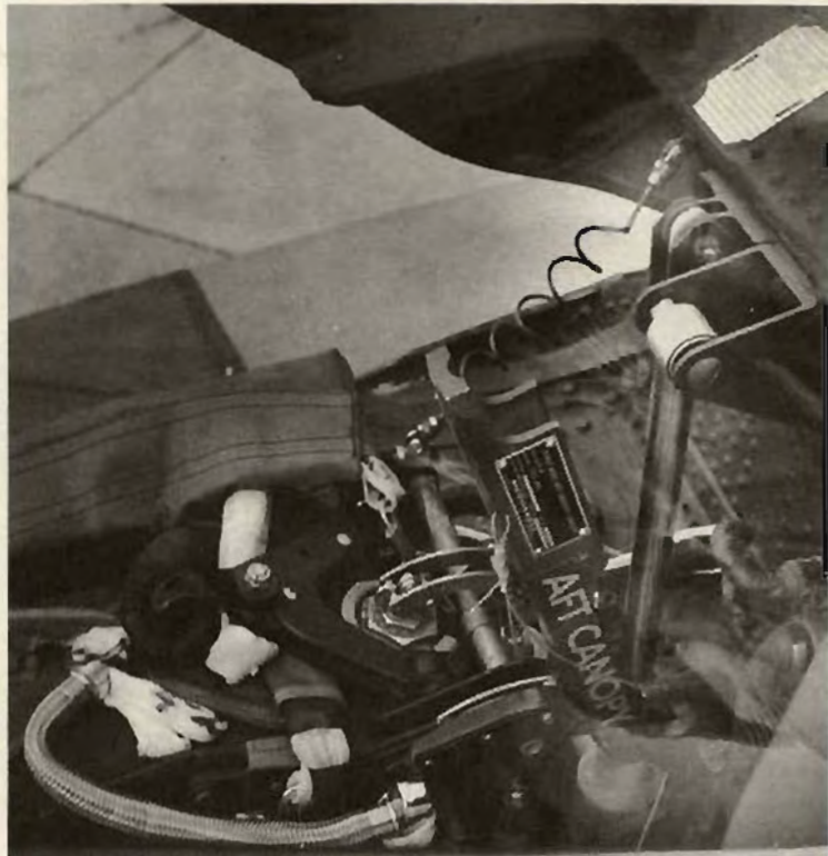
Installing canopy jury struts without inserting locking pin sets up a great booby trap. Upper: Strut can easily teeter forward against banana links. If canopy is closed from ground, or pressure drains off letting it lower, firing mechanism is inevitably damaged. And if Murphy has failed to insert safety pin, the seat gun will fire, though interlock remains in position. Below: Simply inserting jury strut pin may save crew chief embarrassment, and pilots life.
